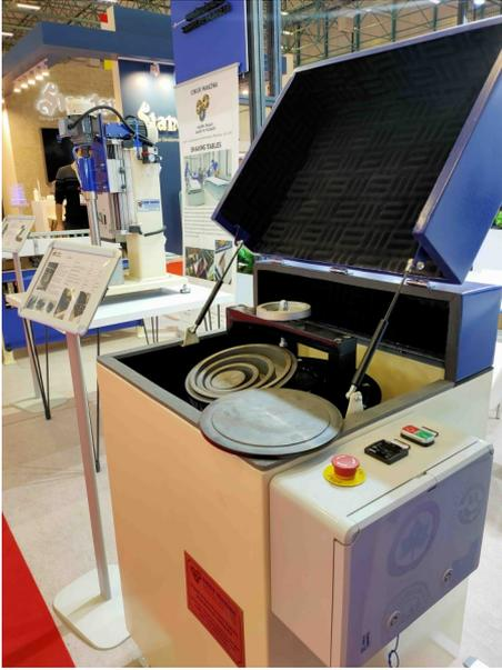
Our HD series Grinding Mills are specifically designed to grind very small materials such as glass, soil, slag, metal oxides, and ceramic materials to obtain the desired particle size.
