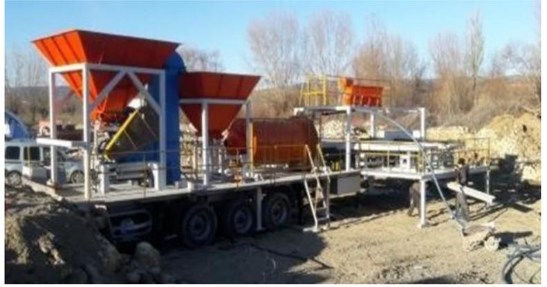
The mobile plant, which includes crushing, grinding, screening, and enrichment units, is designed to be portable. The plant is mounted on wheels and can be easily transported to the mining site with any towing vehicle. The plant provides clean ore recovery with machines that are perfectly integrated with each other.
